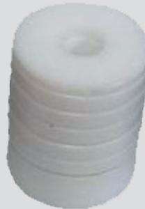
Teflon is virtually impervious to most chemicals and has a wide operating temperature range (-150°C to 230°C).
