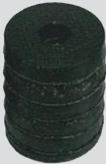
Buna-N is the standard for chemical injection. The most economical and versatile packing, it can be used for methanol, hydrocarbons, ethylene glycol, water, dilute acids, dilute alkali, salt solutions and much more. It is not recommended for keytones, aromatics, polar solvents, etc.
