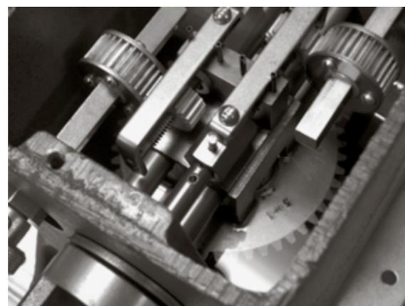
As the shaft is being driven out, care should be taken to see that the large worm gear turns. This will "walk" or disengage the gear teeth. As the shaft emerges from the side of housing, it will force out the oil seal (ASA-2064), seal cartridge (ASA-4045) and ball bearing (ASA-2285). Withdraw the shaft from pump housing.
