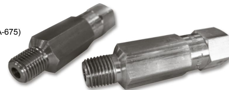
*A line check should be installed in the discharge line as close to the point of injection as possible to prevent backup and contamination of chemical.*
