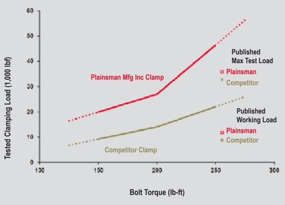
\*Based on actual test results with calibrated equipment, new 1-1/4" single bolt clamps, and new polished rods
